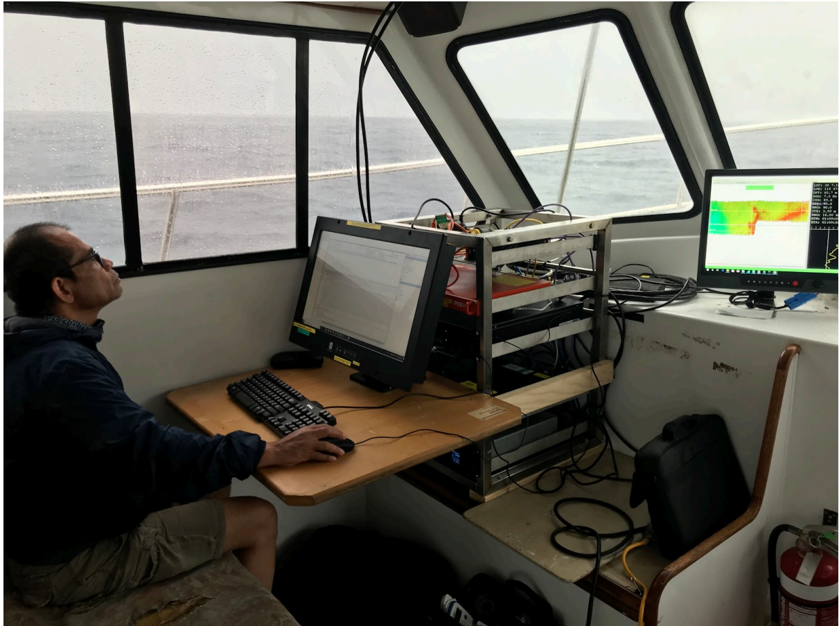
Figure 40 Multibeam sonar acquisition workstation on board FV Santosha.
