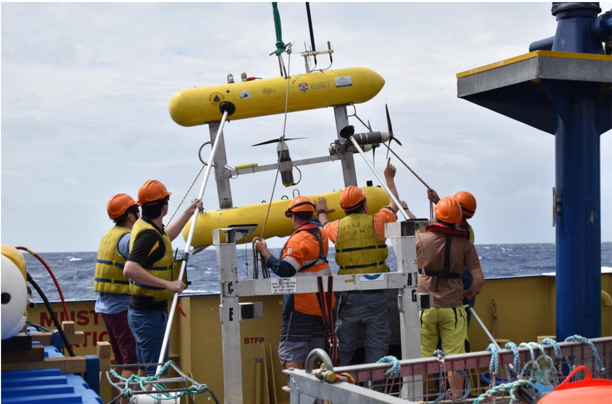
Figure 8. Top image: Deployment of AUV *Sirius* from *TV Bluefin*. Bottom image: Pre-deployment checks of the newly commissioned AUV *Nimbus* by ACRF team (Source: Kristy Brown, IMAS).
