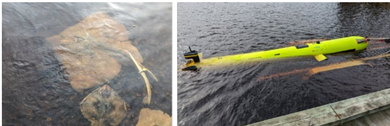
Figure 4-2 (Left) Proxy targets used to simulate Maugean skate across all equipment trials. (Right) REMUS autonomous vehicle with LiDAR and SAS sensor arrays used in Macquarie Harbour for in-situ trials
