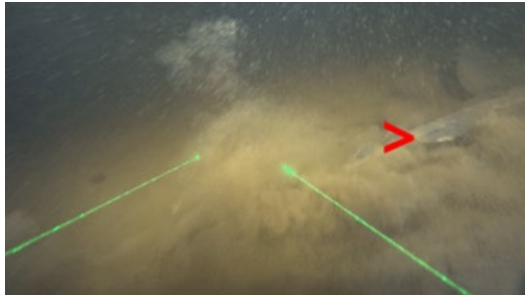
Figure 4-5 Example still frame from traditional towed video trials using external lights in Pine cove Macquarie Harbour at ~12 m depth. A skate can be seen, although due to the small visible area (~0.25 m 2 ) it is not possible to identify the species. Distance between lasers = 20cm
